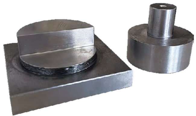
Cross section of a multi-material sprue bushing preform with a fully-printed bushing (right).
