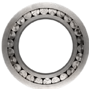
Assembled bearing with nickel rings and cobalt rollers.
